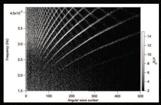
I-v diagram computed from three days of SODISM solar observations at 535 nm (limb images in April 2011).
